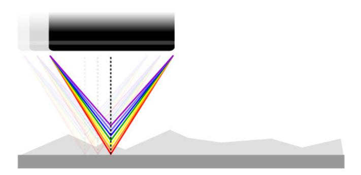
Nanovea optical pens have zero influence from sample reflectivity. Variations require no sample preparation and have advanced ability to measure high surface angles. Capable of large Z measurement ranges. Measure any material: transparent/opaque, specular/diffusive, polished/rough. Measurement includes: Profile Dimension, Roughness Finish Texture, Shape Form Topography, Flatness Warpage Planarity, Volume Area, Step-Height Depth Thickness and many others.
